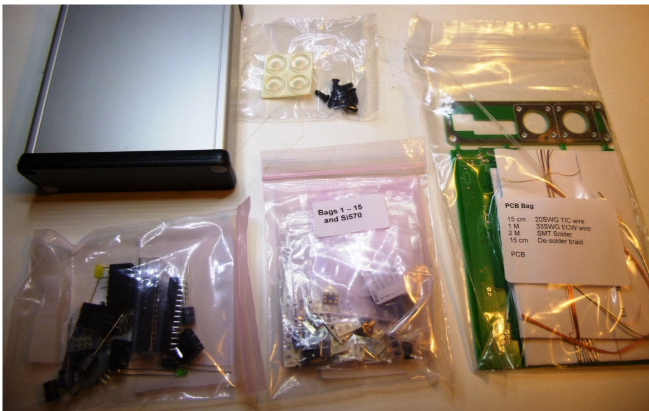
The Hunter SDR kit comes as a number of parts - Don't mix the bags, the capacitors have no labels!
