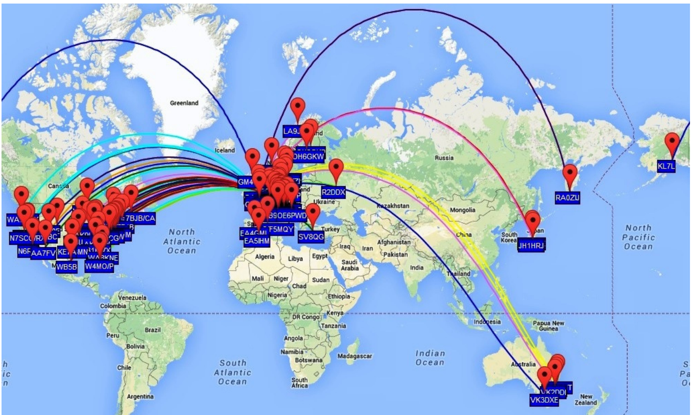
Stations Worked in One Day Using WSPR - Power level 1 Watt
